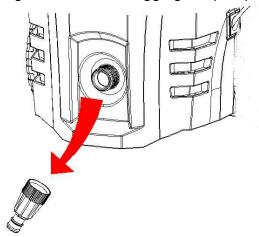
Clean the nozzle with the needle clean-out tool provided. Remove the spray wand from the gun. Remove any dirt from the nozzle hole and rinse.
