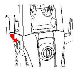
4. Slide the power cord hook into position of unit right.
